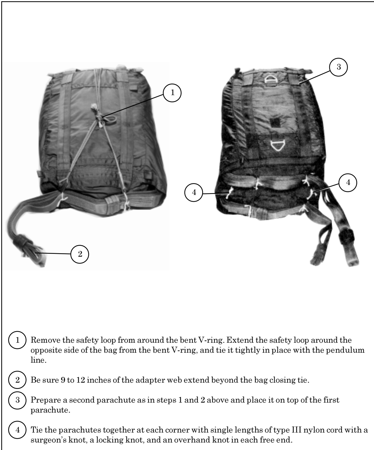
Figure 3-69. Clustering Extraction Parachutes for a Sequential Extraction
